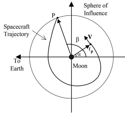
Fig. 1 – Parameters of the gravitational capture.
