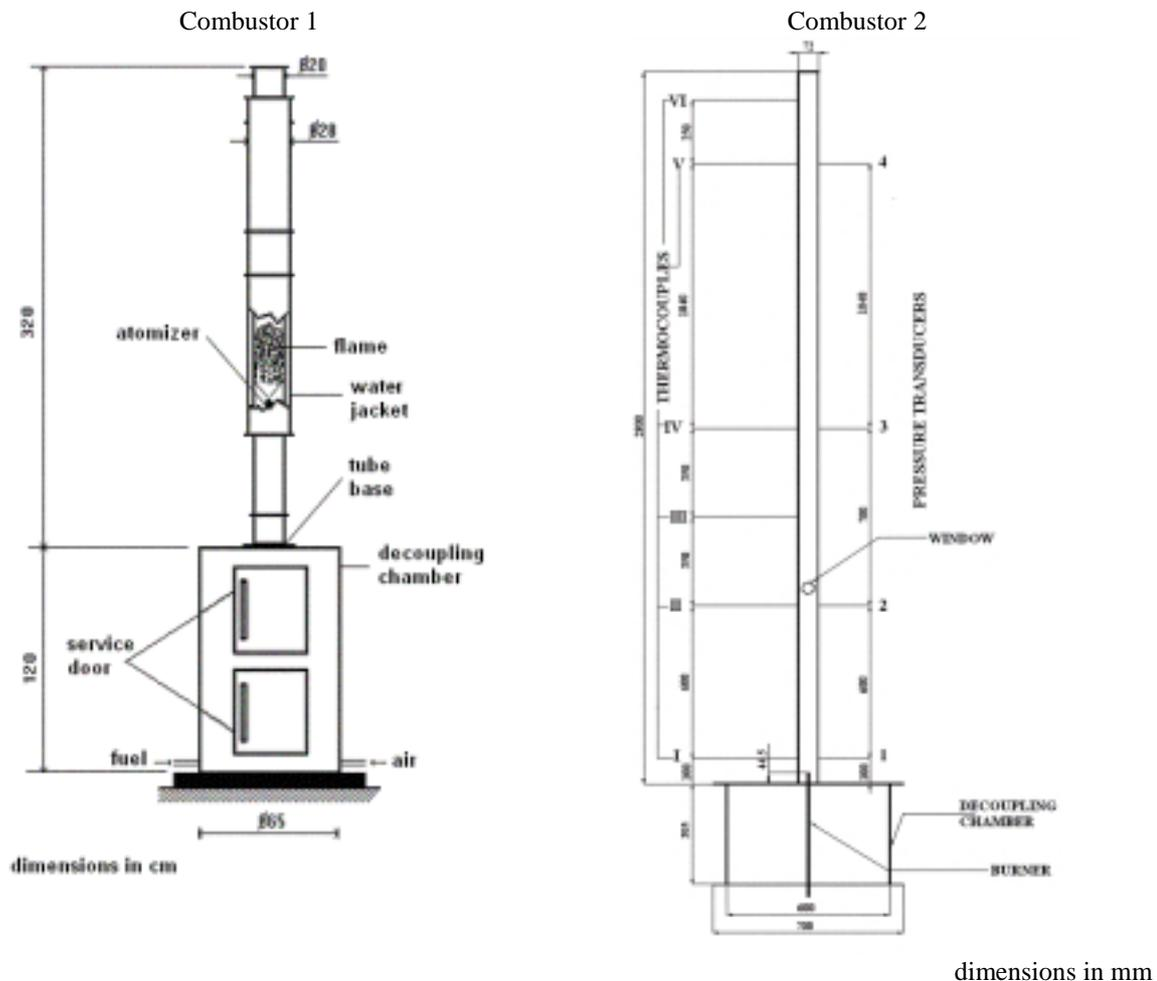
Figure 2 - Schematic diagrams for both Rijke tube combustors.
