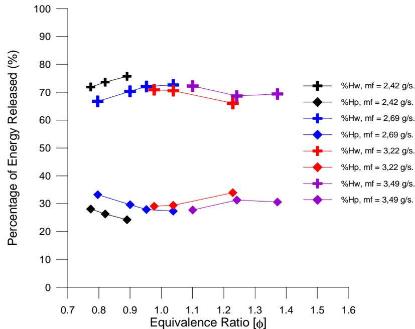
Figure 5 - Results of the energy balance for the testes described in Tab. (3)<sup>1</sup>.
