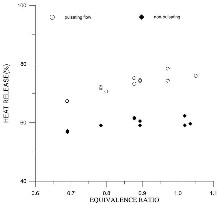
Figure 7. Percentage of the heat release to the water (fuel rate of the 0.30 g/s)
