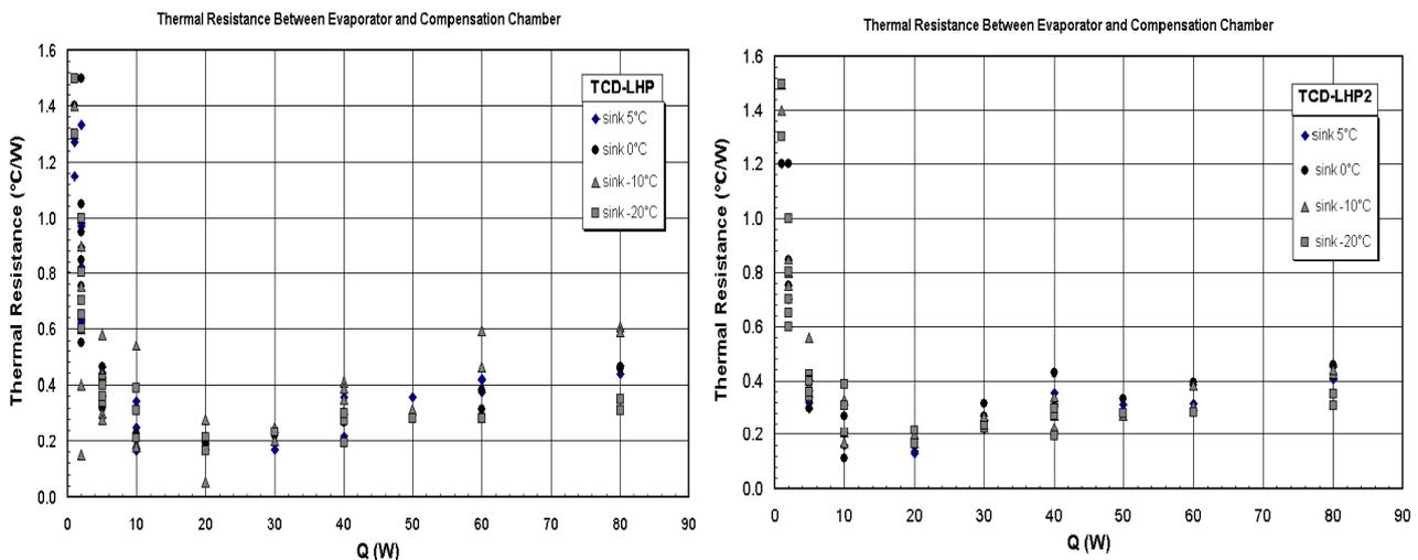
Figure 5. Overall results of the thermal resistances.
