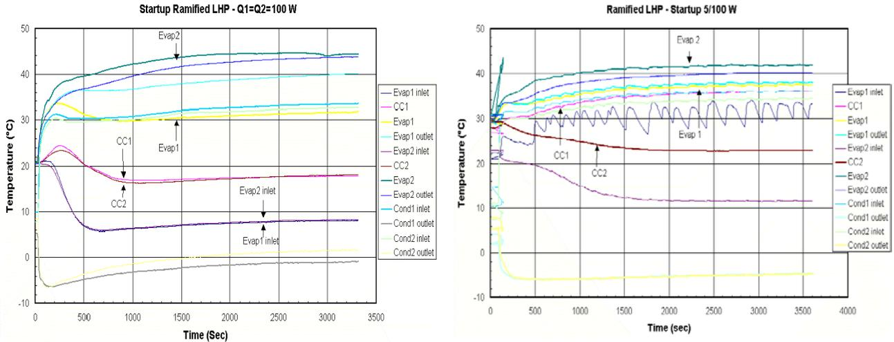
Figure 9. Startup procedures of the ramLHP.
