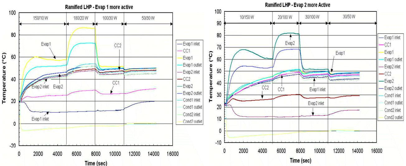
Figure 10. Power cycle applied to the ramLHP.
