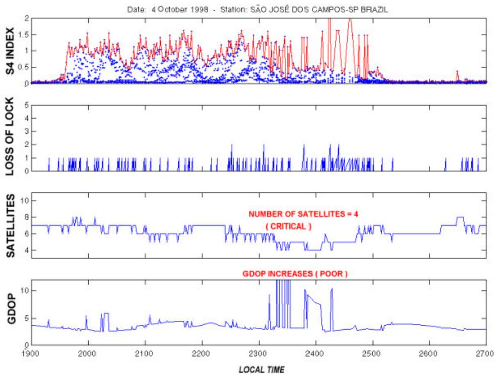
Figure 14- Example of losses of lock, increase in the dilution of precision and decrease in the number of available GPS satellites during ionospheric scintillations
