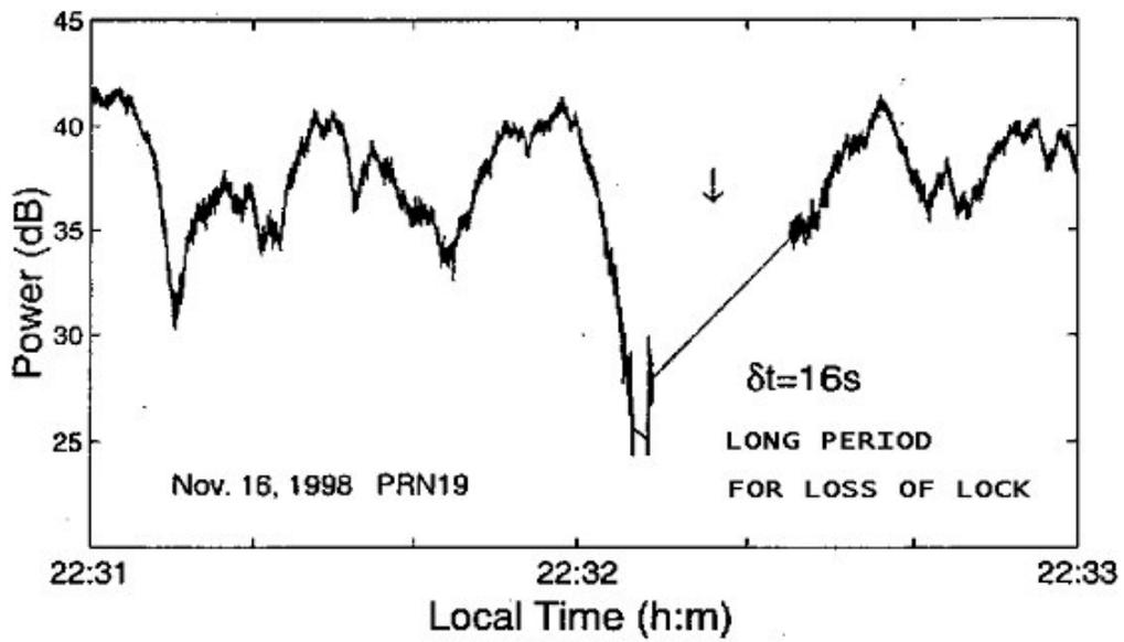
Figure 13- Example of losses of lock during ionospheric irregularities. Source: Kintner et al. (2001)
