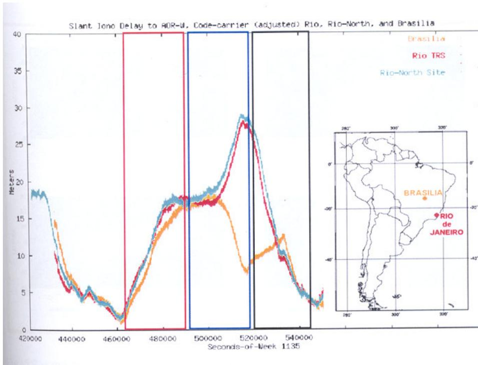
Figure 2- The effects of the Total Electron Content (TEC) over GPS signal under the Equatorial Ionospheric Anomaly region. Source: Tom Dehel ( FAA – Federal Aviation Administration – USA ), 2002
