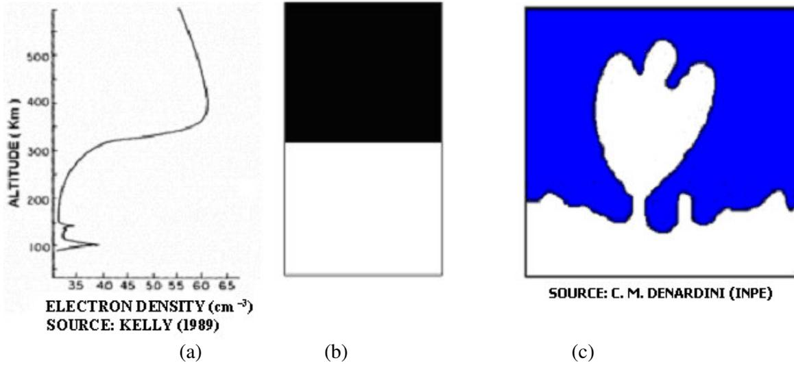
Figure 4- Ionospheric electron density profile with a large gradient around 360 Km ( a ); illustration of a heavier plasma resting over the neutral atmosphere (b); and the illustration of one bubble after its generation and evolution (c)
