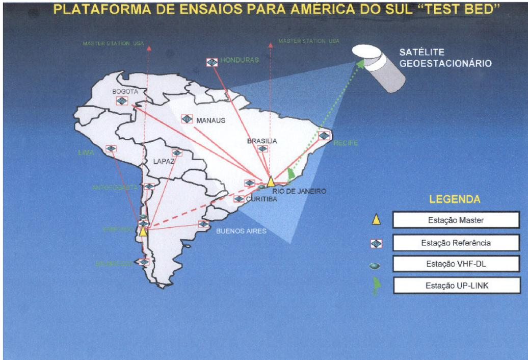
Figure 15- Brazilian Space Based Augmentation System (SBAS) test bed
