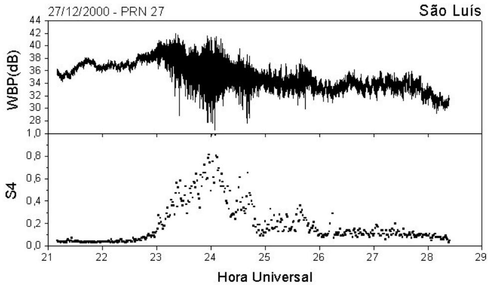
Figure 12- Example of GPS ionospheric scintillations during the occurrence of ionospheric scintillations represented by the S4 scintillation index. Source: Rodrigues ( 2003 )
