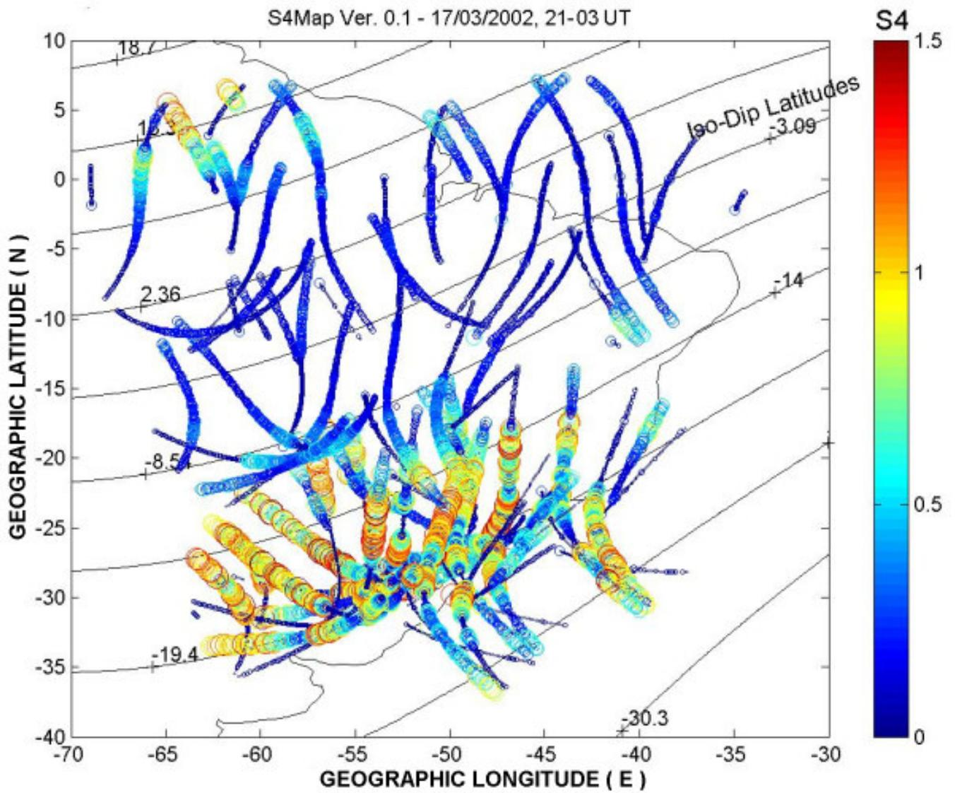
Figure 6- Ionospheric scintillations represented by the S4 scintillation index, during March 17, 2002, over Brazil. Source: Rodrigues ( 2003 )
