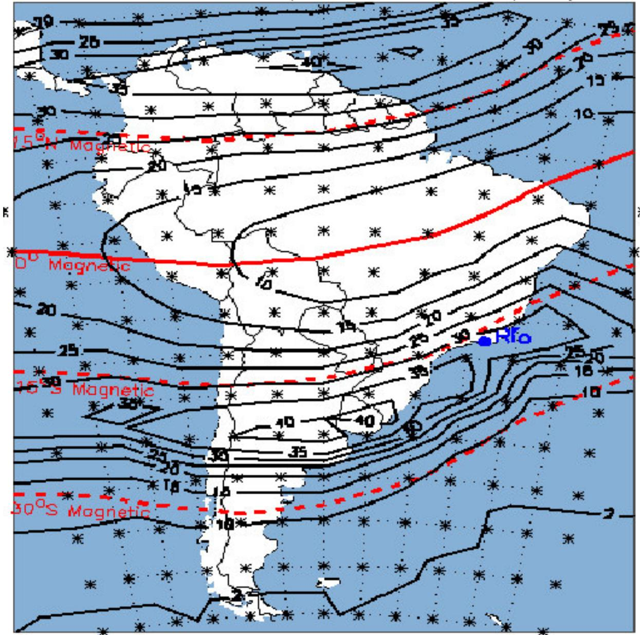
Figure 3- GPS vertical ionospheric delays due to TEC over South America calculated using a low latitude ionospheric model. Source: Klobuchar et al. ( 2002 )
