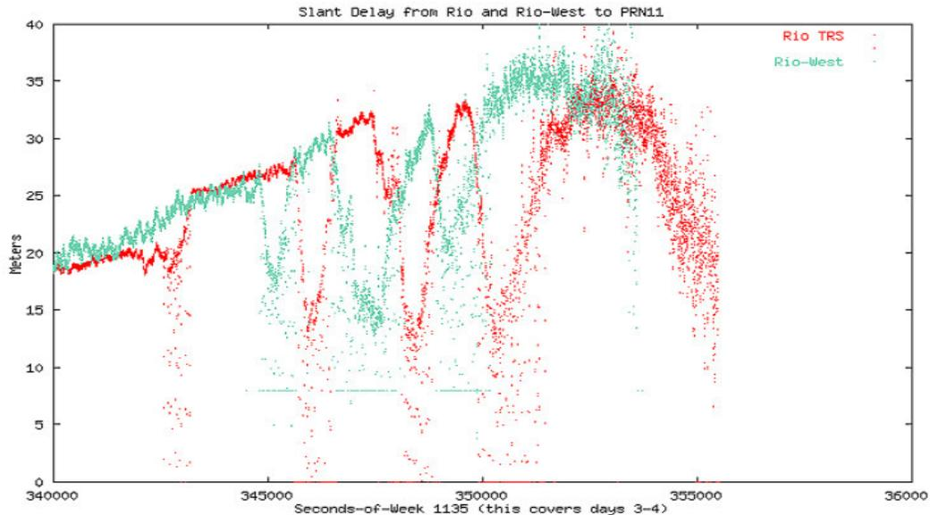
Figure 10- GPS slant delays at Rio de Janeiro associated with large TEC depletions due to the ionospheric irregularities. Source: Tom Dehel ( 2002 )
