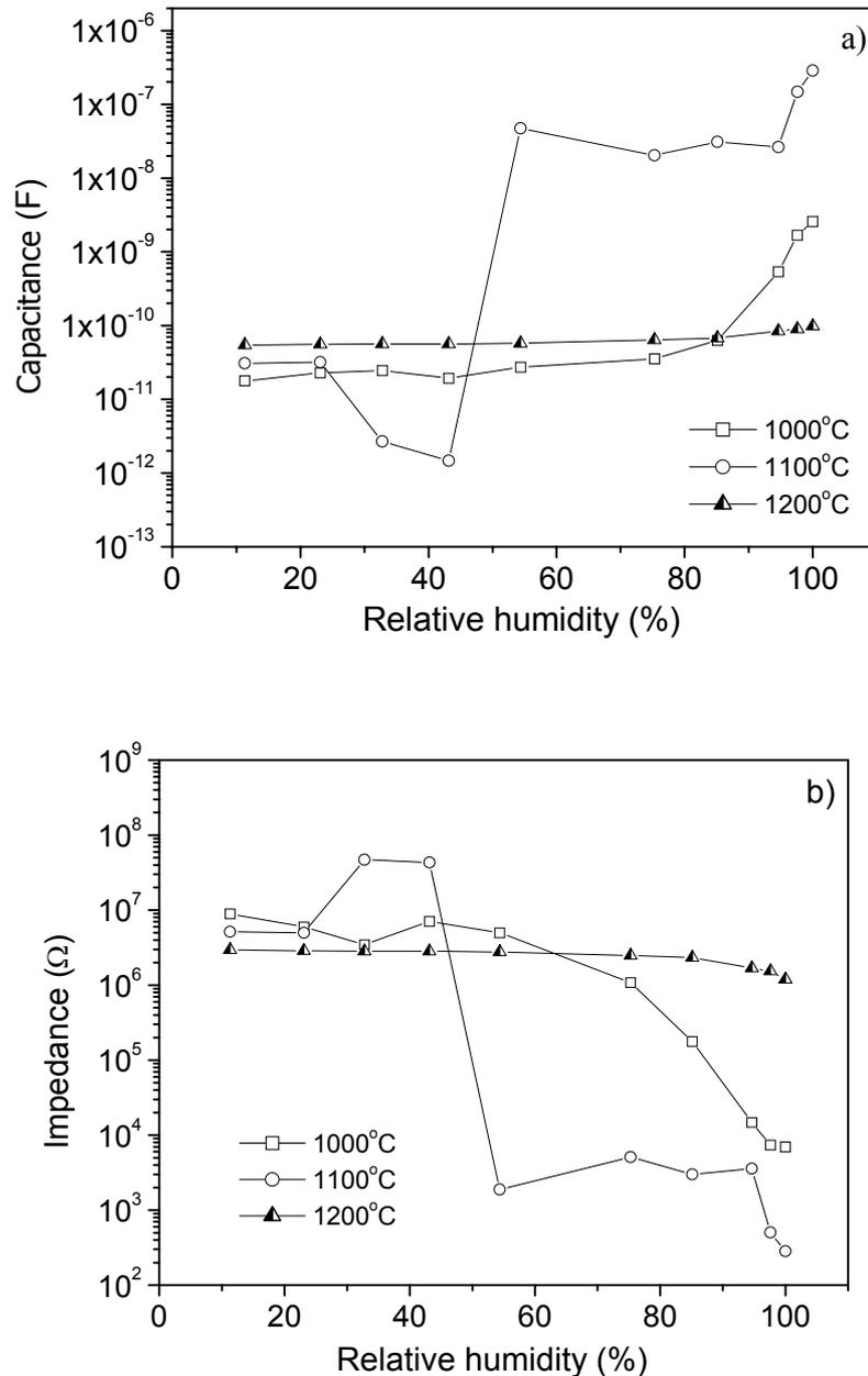
Figure 5 Dielectric properties according to change in relative humidity for ZnO<sub>2</sub>-TiO<sub>2</sub>-Ta<sub>2</sub>O<sub>5</sub> ceramic: a) impedance and b) capacitance measures.
