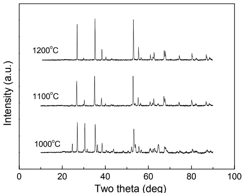
Figure 1 X-ray diffraction patterns of  $\text{ZnO}_2$ - $\text{TiO}_2$ - $\text{Ta}_2\text{O}_5$  sintered ceramics.
