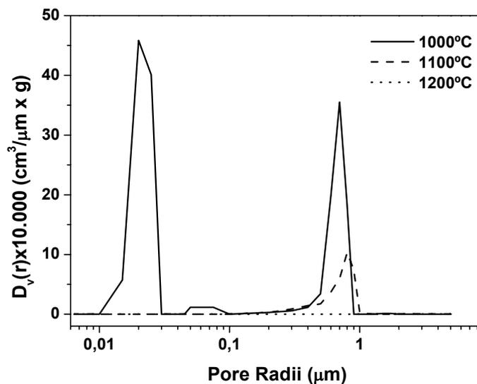
Figure 3 Pore size distribution curves of the sintered ceramics calculated from the mercury porosimetry data.
