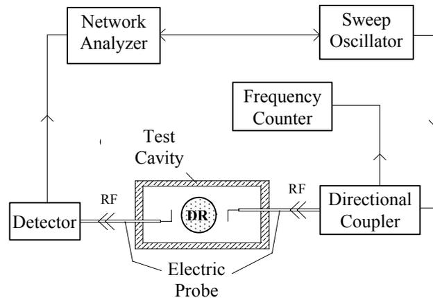
Figure 2. Experimental setup for measuring the microwave parameters
