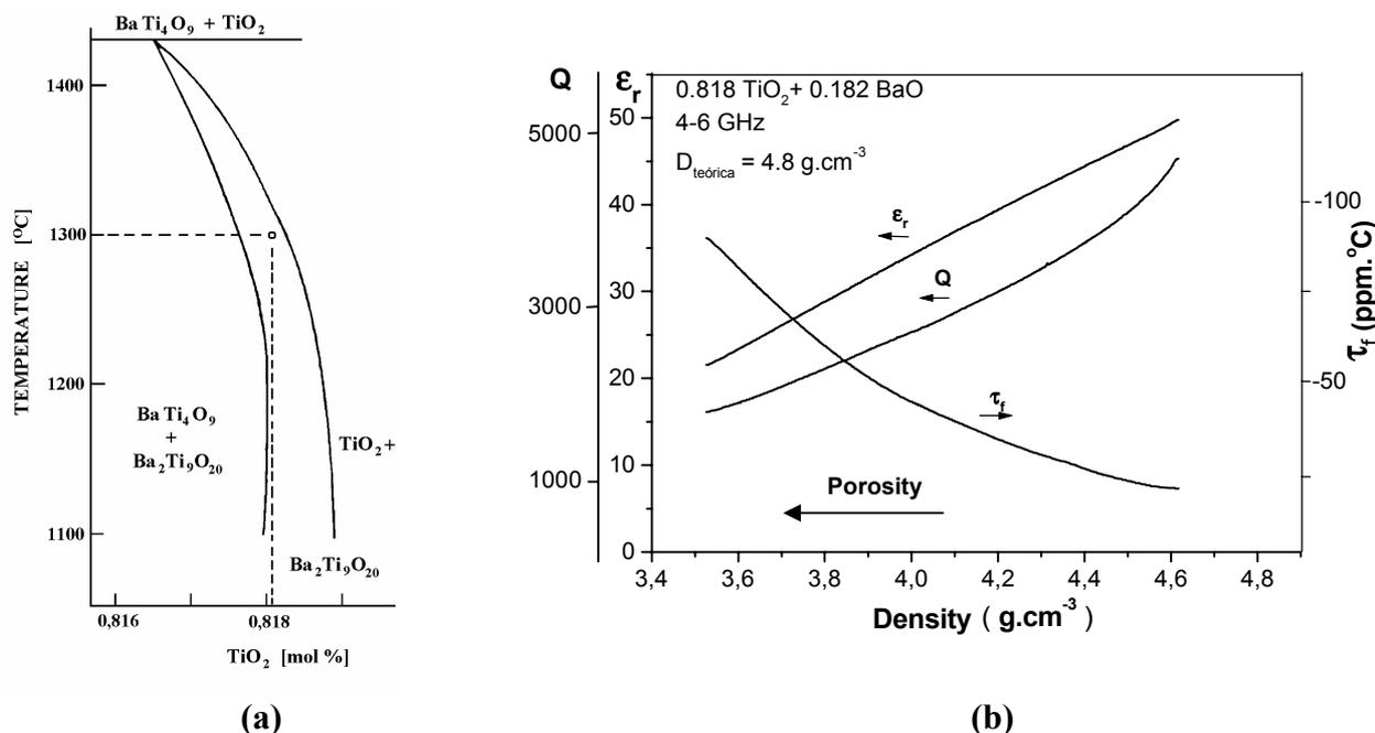
Figure 1. (a) Phase equilibrium diagram for  $\text{Ba}_2\text{Ti}_9\text{O}_{20}$  region from 1100 to 1400°C of the system BaO-TiO<sub>2</sub> [1] and (b) effect of density on the dielectric characteristics of  $\text{Ba}_2\text{Ti}_9\text{O}_{20}$  ceramic [1,5]
