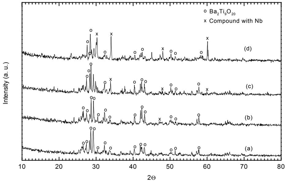
Figure 3. X-ray diffraction patterns for the investigated ceramics: (a) Trans-Tech DR, (b) without Nb addition, (c) with 0.2 mol % Nb, and (d) with 0.4 mol % Nb
