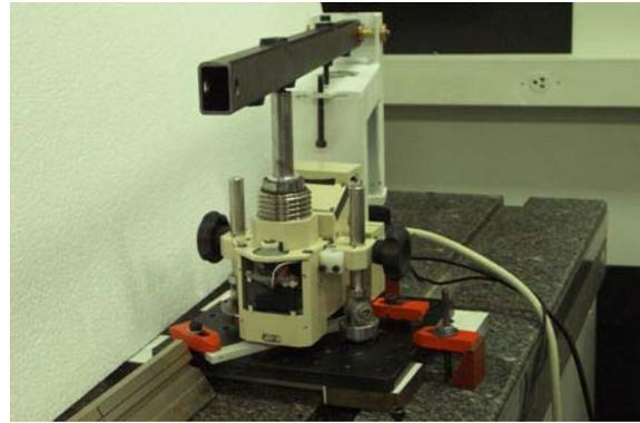
Figure 4.2 Preliminary indentation system and the radial interferometer.
