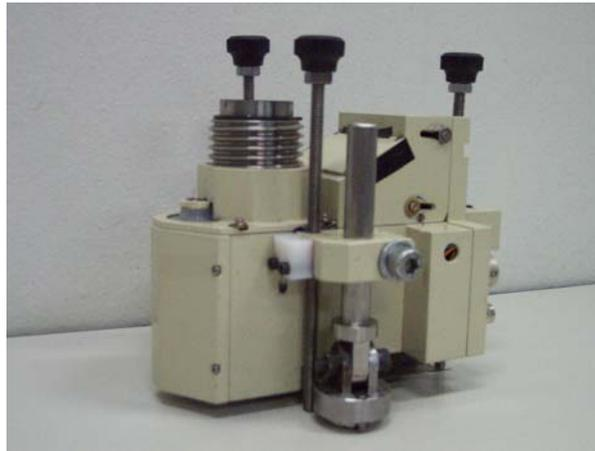
Figure 4.1 ESPI residual stress measurement (MTRES).
