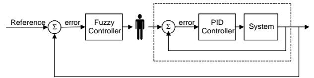
Figure 4 - Inner and Outer Control Action
