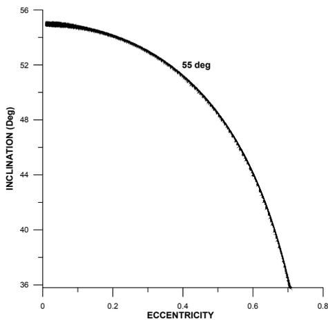
Fig. 15. Eccentricity vs. Inclination for  $i(0) = 55 \text{ deg}$ .
