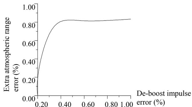
**Fig. 5 Extra-atmospheric range changes related to value of de-boost impulse error**
