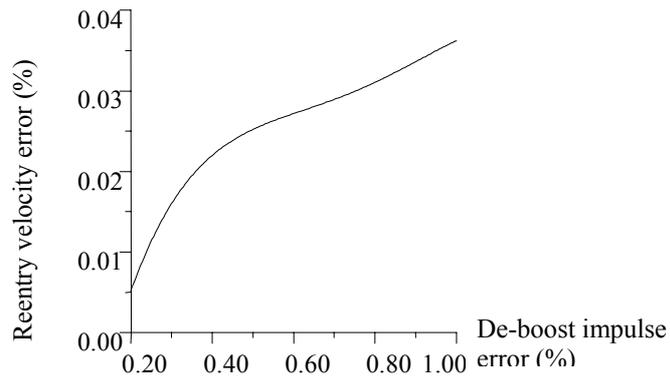
**Fig. 3 Re-entry velocity changes related to value of de-boost impulse error**
