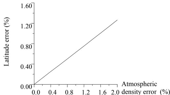
**Fig. 6 Latitude disturbance related to atmospheric density error**
