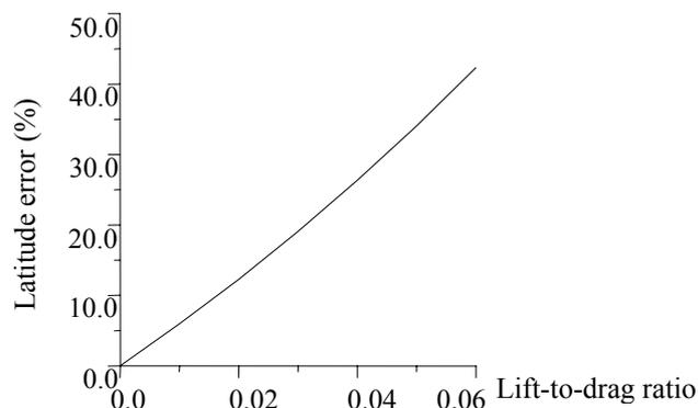
**Fig. 10 Latitude disturbance related to lift-to-drag ratio**
