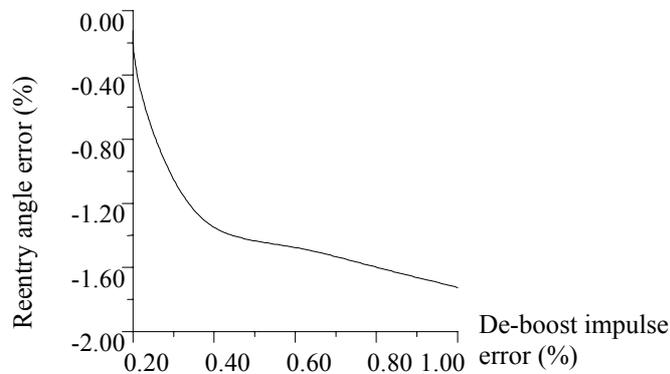
**Fig. 4 Re-entry angle changes related to value of de-boost impulse error**
