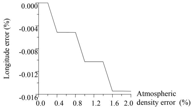
**Fig. 7 Longitude disturbance related to atmospheric density error**
