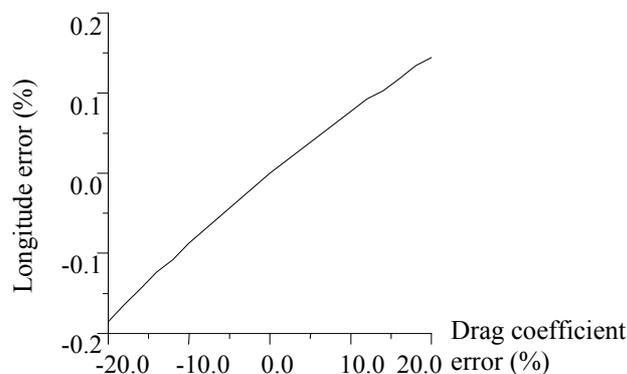
**Fig. 9 Longitude disturbance related to drag coefficient error**
