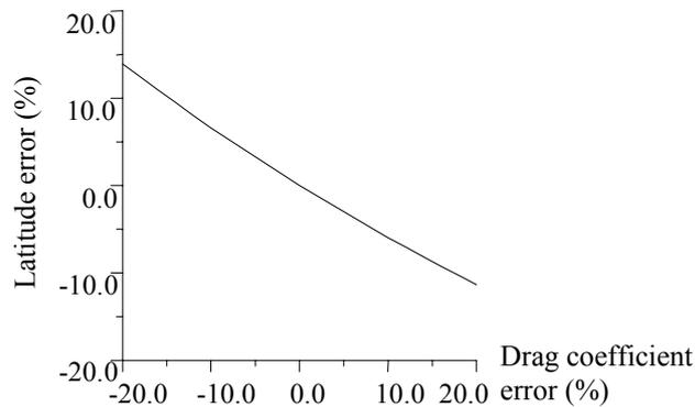
**Fig. 8 Latitude disturbance related to drag coefficient error**
