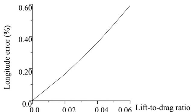
**Fig. 11 Longitude disturbance related to lift-to-drag ratio**
