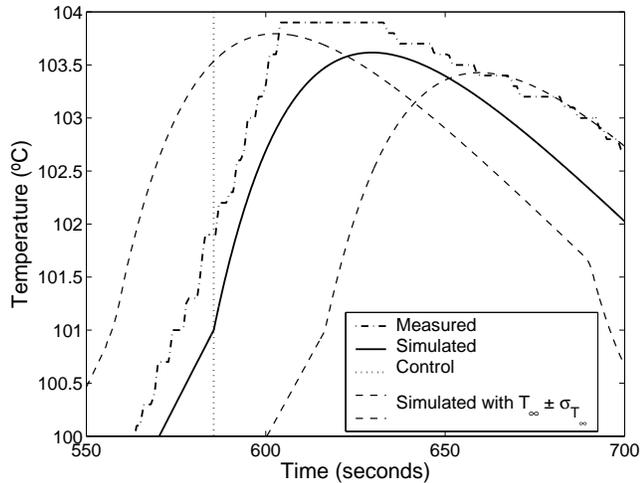
Figure 3 – Simulation realized varying the parameter  $T_{\infty}$
