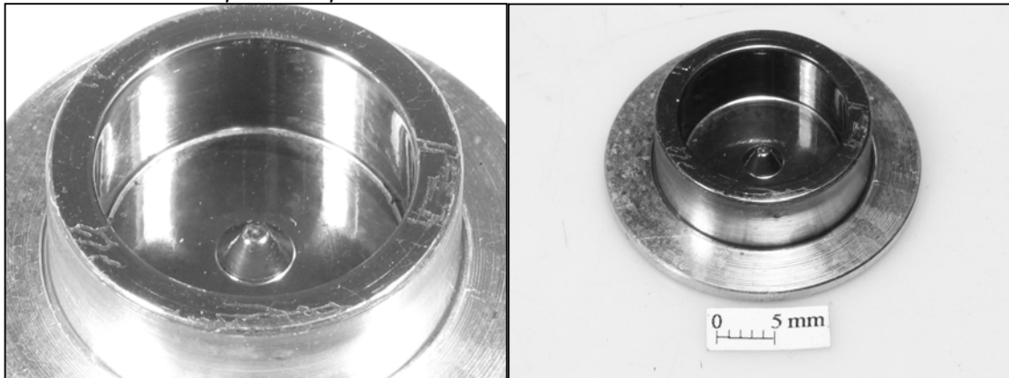
Figure 3 - Copper-aluminum klystron cavity covered with a thin layer of niobium.
