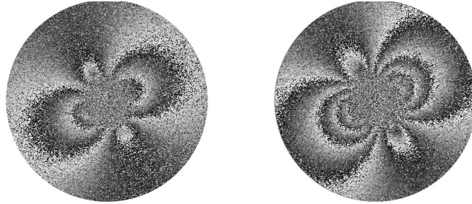
Figure 2: Typical phase difference patterns for two different residual stresses levels.
