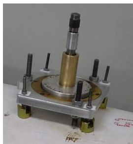
Figure 5: Indentation module with a 120° conical diamond or a 2.5 mm diameter spherical tungsten carbide tips.
