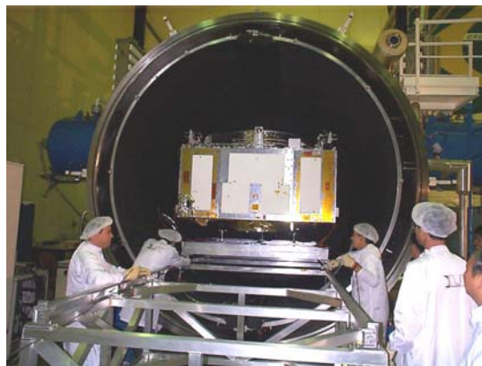
Figure 5. Preparation for Global Leak Tests - INPE
