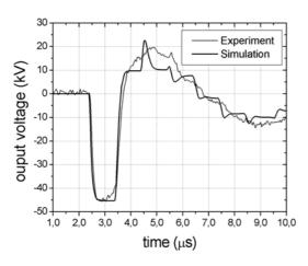
Figure 9. Experimental and simulated output voltages shown in an expanded time scale.
