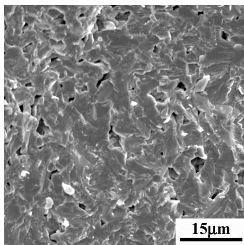
Figure 4. SEM micrographs of  $Ba_2Ti_9O_{20}$  ceramic fracture surfaces from Trans-Tech
