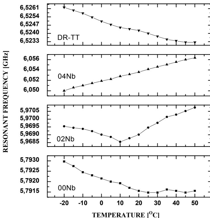
Figure 6. Measurements of resonant frequency variation with temperature in the range  $-20^{\circ}\text{C}$  to  $+50^{\circ}\text{C}$  for DRs referred in Table 1
