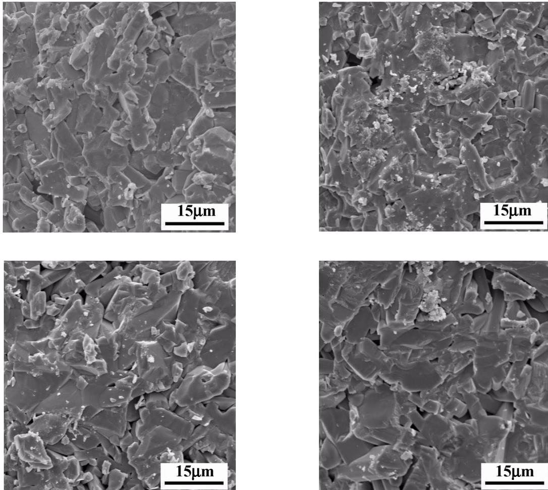
Figure.5 SEM micrographs of  $\text{Ba}_2\text{Ti}_9\text{O}_{20}$  ceramic fracture surfaces: a) without  $\text{Nb}_2\text{O}_5$  addition, b) with 0.1 mol%  $\text{Nb}_2\text{O}_5$ , c) with 0.2 mol%  $\text{Nb}_2\text{O}_5$  and d) with 0.4 mol%  $\text{Nb}_2\text{O}_5$
