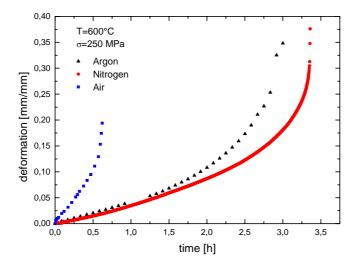
Figure 3 - Creep curves at 600°C and 250MPa obtained in argon, nitrogen and air atmospheres.
