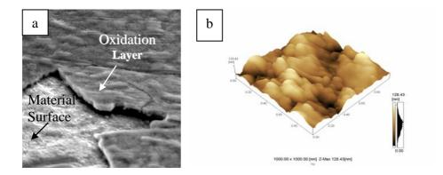
Figure 2 - Microstructure of oxidation layer by SEM (a) and surface roughness obtained by AFM (b).
