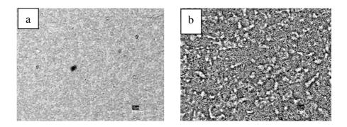
Figure 1 - Microstructures obtained by SEM of one sample without treatment (a) and one treated at  $600^{\circ}$ C in air atmosphere (b).
