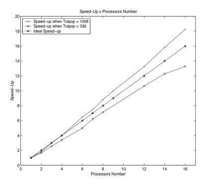
Figure 3: Speed-up versus the number of processors considering the two population sizes
