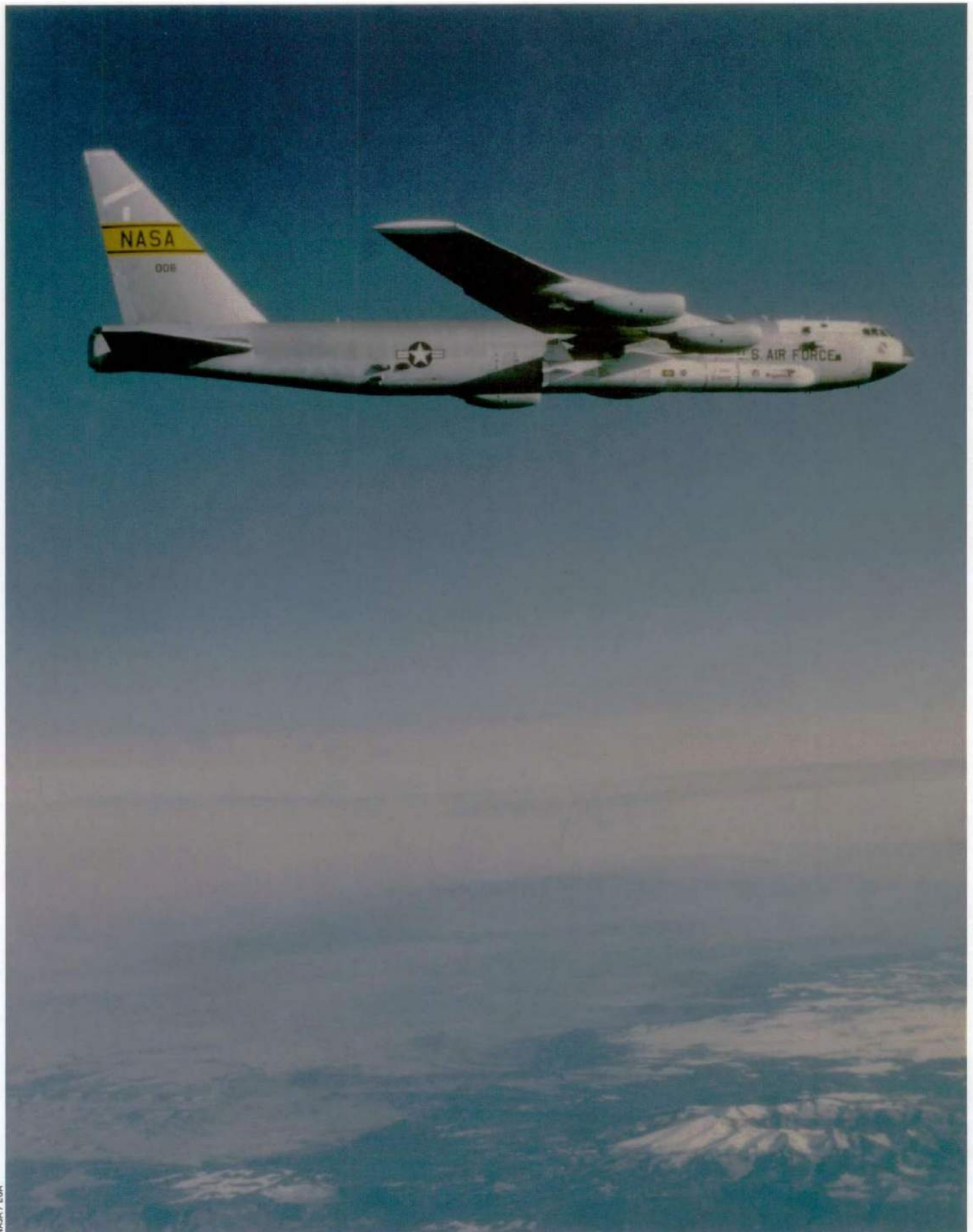
O avião B-52 em voo, levando o Pegasus com o SCD-1 B-52 in flight, carrying the Pegasus launch vehicle with the SCD-1 satellite.
