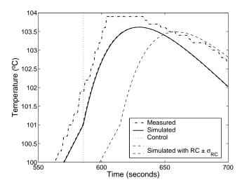
Figure 4 – Simulation realized varying the parameter RC
