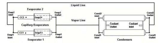
Figure 8. Representation of the ramified LHP test bed.
