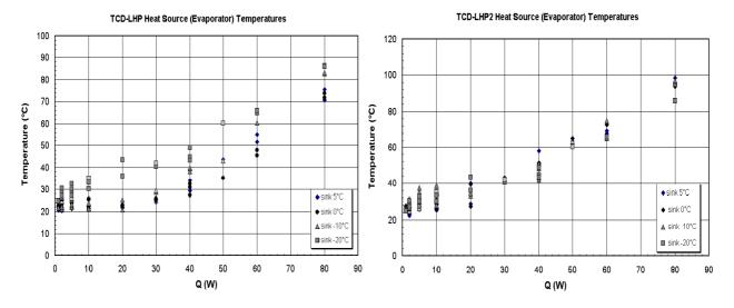
Figure 4. Overall results of the heat source temperatures.
