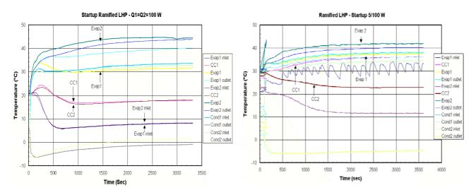
Figure 9. Startup procedures of the ramLHP.
