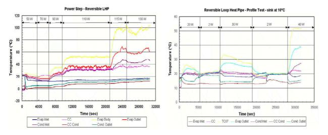
Figure 7. Power step and profile test with the r-LHP.
