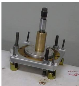
Figure 5: Indentation module with a 120° conical diamond or a 2.5 mm diameter spherical tungsten carbide tips.
