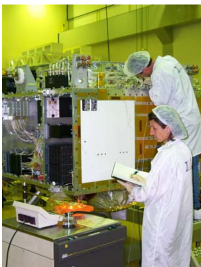
Figure 4. Local Leak Tests - INPE
