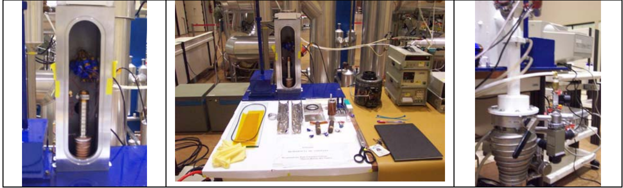
Figure 2. High Vacuum Chamber: the specimen with heat source (skin-heater) installed in a cold serpentine, and thermocouples (left side); General View of the test setup (center); Vacuum Pumping System (right side).
