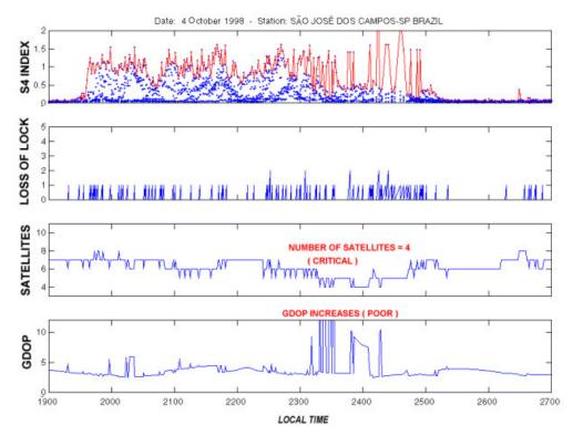
Figure 14- Example of losses of lock, increase in the dilution of precision and decrease in the number of available GPS satellites during ionospheric scintillations
