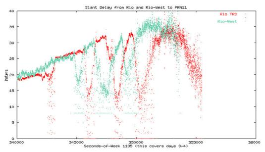
Figure 10- GPS slant delays at Rio de Janeiro associated with large TEC depletions due to the ionospheric irregularities. Source: Tom Dehel (2002)
