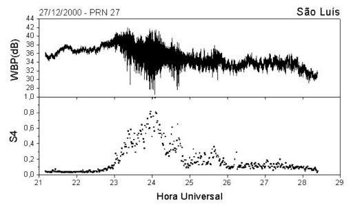
Figure 12- Example of GPS ionospheric scintillations during the occurrence of ionospheric scintillations represented by the S4 scintillation index. Source: Rodrigues (2003)
