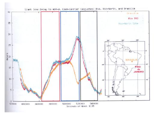
Figure 2- The effects of the Total Electron Content (TEC) over GPS signal under the Equatorial Ionospheric Anomaly region. Source: Tom Dehel (FAA – Federal Aviation Administration – USA), 2002
