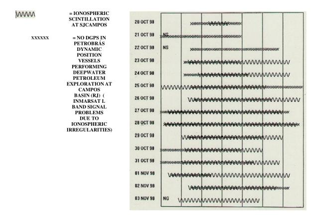
Figure 16- Effects of the ionospheric irregularities over DGPS (differential) system. Source: de Paula et al. (1999)
