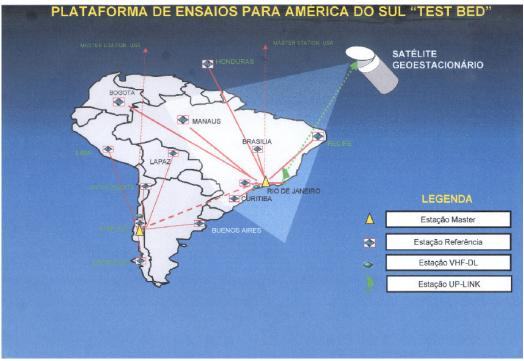
Figure 15- Brazilian Space Based Augmentation System (SBAS) test bed
