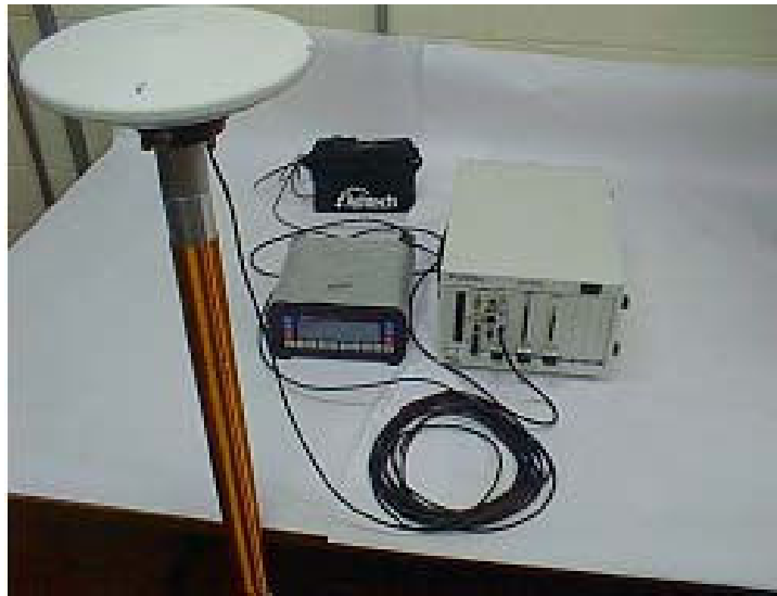
Figure 2. GPS antenna, Z-12 receiver, battery and computer
