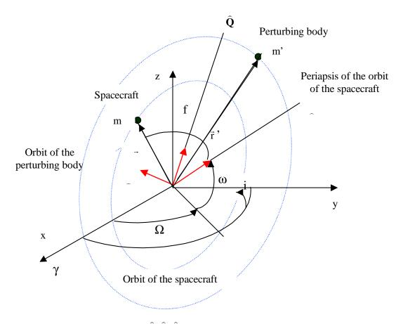
Fig. 2. The orthogonal set  $\hat{\mathbf{P}}$ ,  $\hat{\mathbf{Q}}$ ,  $\hat{\mathbf{R}}$  and the coordinate system in the orbital plane.
