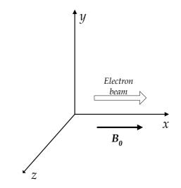
Figure 1 - Reference system used in our simulation. It shows an electron beam propagating parallel to the background magnetic field, both in the x -direction of the system.
