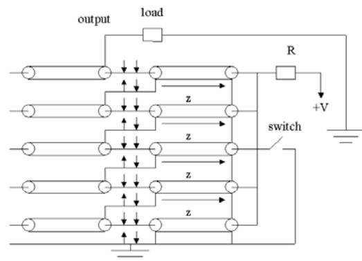
Figure 1. A coaxial Blumlein pulser made of 10 lines.
