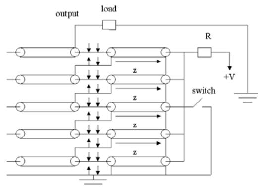
Figure 1. A coaxial Blumlein pulser made of 10 lines.
