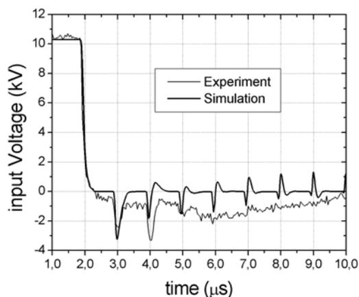
**Figure 8.** Experimental and simulated input voltages shown in an expanded time scale.
