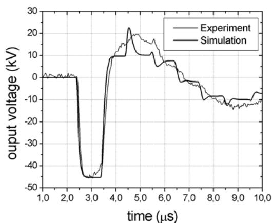
**Figure 9.** Experimental and simulated output voltages shown in an expanded time scale.
