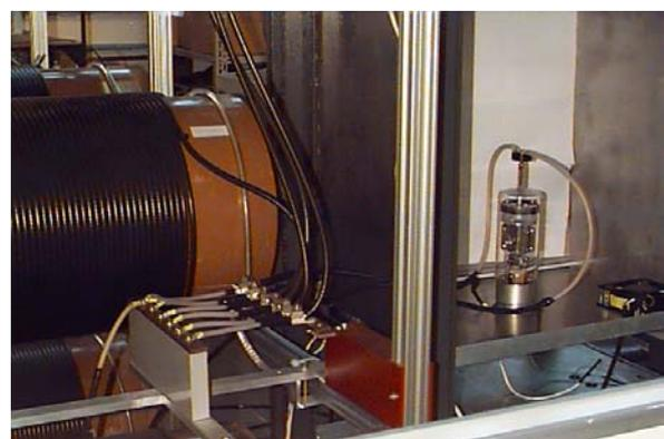
**Figure 4.** Picture showing the coaxial input connection.
