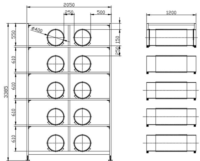
**Figure 2.** Pulser sectional cross view in mm.
