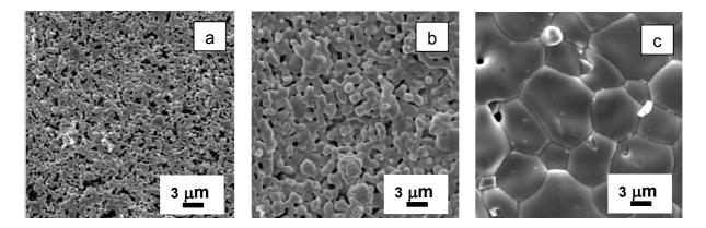
Figure 4 SEM micrographs of ZnO<sub>2</sub>-TiO<sub>2</sub>-Ta<sub>2</sub>O<sub>5</sub> ceramics sintered at 1000°C (a), 1100°C (b) and 1200°C (c).
