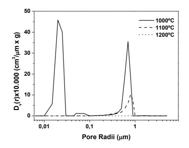
Figure 3 Pore size distribution curves of the sintered ceramics calculated from the mercury porosimetry data.
