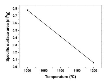
Figure 2 Specific surface area for the ZnO<sub>2</sub>-TiO<sub>2</sub>-Ta<sub>2</sub>O<sub>5</sub> sintered ceramics measured by BET nitrogen adsorption.
