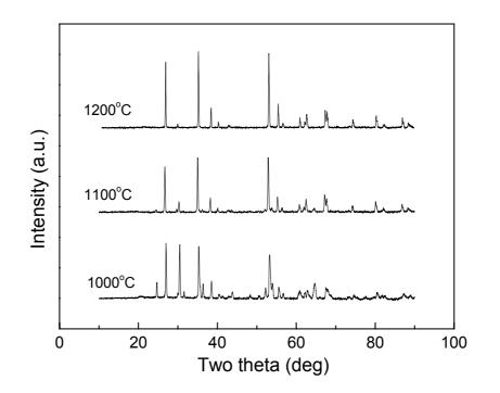
Figure 1 X-ray diffraction patterns of ZnO<sub>2</sub>-TiO<sub>2</sub>-Ta<sub>2</sub>O<sub>5</sub> sintered ceramics.
