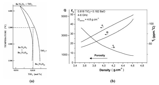
Figure 1. (a) Phase equilibrium diagram for  $Ba_2Ti_9O_{20}$  region from 1100 to 1400°C of the system  $BaO-TiO_2$  [1] and (b) effect of density on the dielectric characteristics of  $Ba_2Ti_9O_{20}$  ceramic [1,5]
