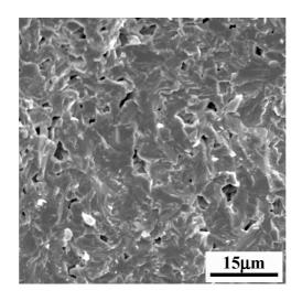
Figure.4. SEM micrographs of Ba<sub>2</sub>Ti<sub>9</sub>O<sub>20</sub> ceramic fracture surfaces from Trans-Tech
