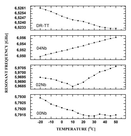
Figure 6. Measurements of resonant frequency variation with temperature in the range -20°C to +50°C for DRs referred in Table 1
