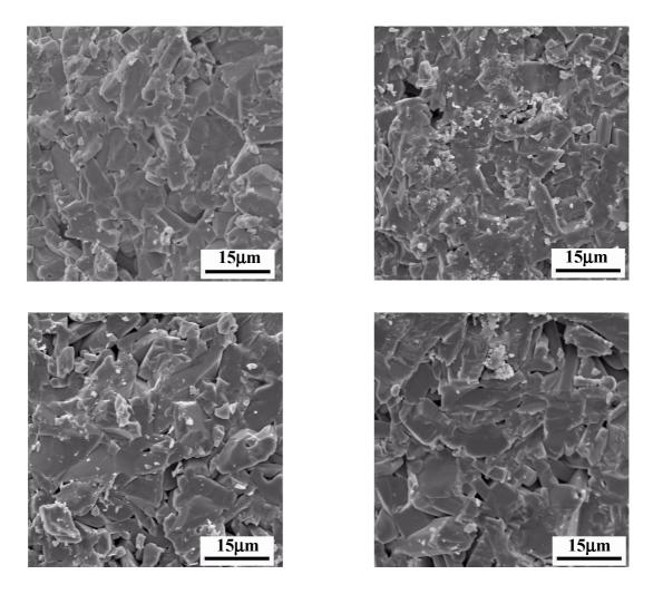
Figure.5 SEM micrographs of Ba<sub>2</sub>Ti<sub>9</sub>O<sub>20</sub> ceramic fracture surfaces: a) without Nb<sub>2</sub>O<sub>5</sub> addition, b) with 0.1 mol% Nb<sub>2</sub>O<sub>5</sub>, c) with 0.2 mol% Nb<sub>2</sub>O<sub>5</sub> and d) with 0.4 mol% Nb<sub>2</sub>O<sub>5</sub>
