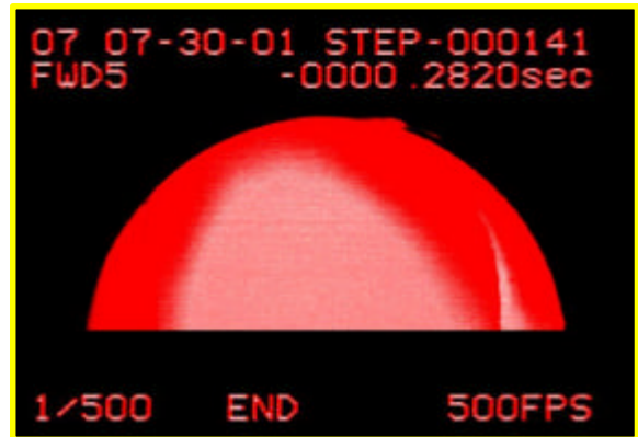
Figure 2. D-shaped plasma picture taken with the CCD camera
