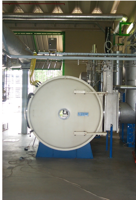
Figure 8. The vacuum chamber used in the tests at INPE-LCP.
