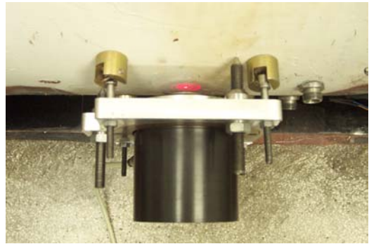
Figure 6 - Experiment in progress (a) interferometer positioned on the pipe (b) a close view of the interferometer
