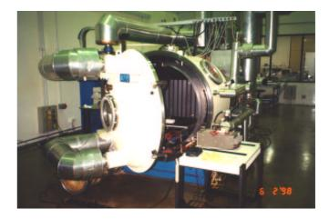
Figure 2 - Thermal-Vacuum Chamber
