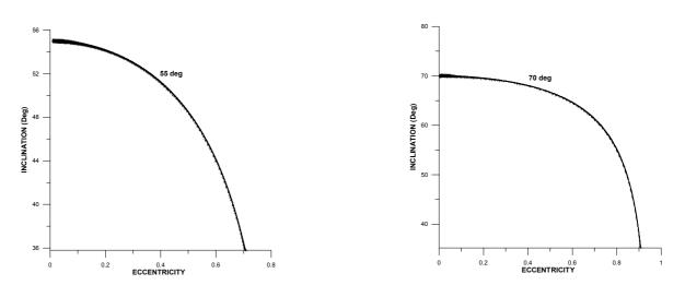
Fig. 15. Eccentricity vs. Inclination for i (0) = Fig. 16. Eccentricity vs. Inclination for i (0) = 55 deg. 70 deg.
