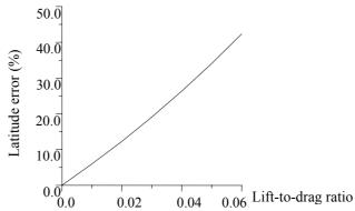
Fig. 10 Latitude disturbance related to lift-to-drag ratio
