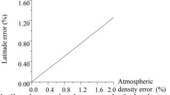
Fig. 6 Latitude disturbance related to atmospheric density error
