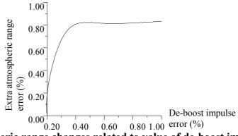
Fig. 5 Extra-atmospheric range changes related to value of de-boost impulse error
