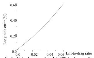
Fig. 11 Longitude disturbance related to lift-to-drag ratio
