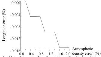
Fig. 7 Longitude disturbance related to atmospheric density error
