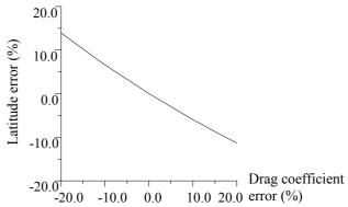
Fig. 8 Latitude disturbance related to drag coefficient error
