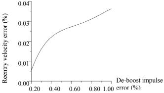
Fig. 3 Re-entry velocity changes related to value of de-boost impulse error
