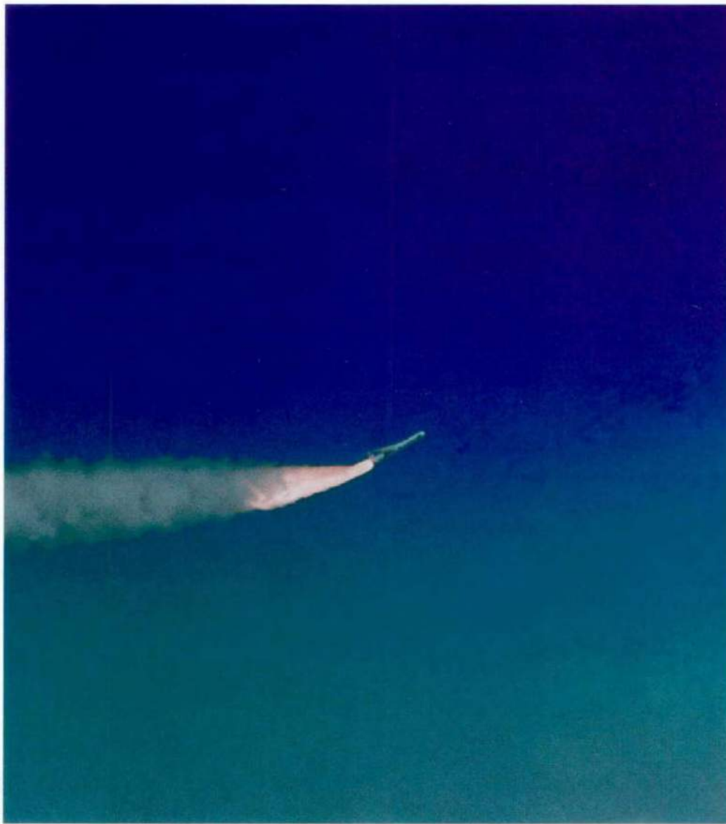
O foguete Pegasus com o SCD-1 a bordo, após ser lançado do avião B-52 da NASA. The Pegasus vehicle, with the SCD-1 satellite aboard, immediately after its release from the B-52.
