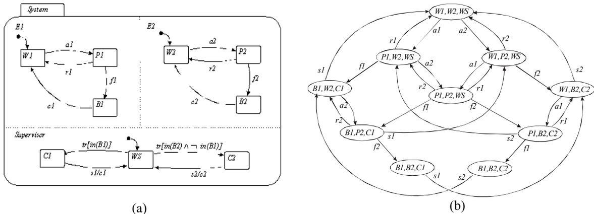
Figure 1. Statecharts representation. (a) System with two machines and a repairer; (b) Resulting Markov Chain
