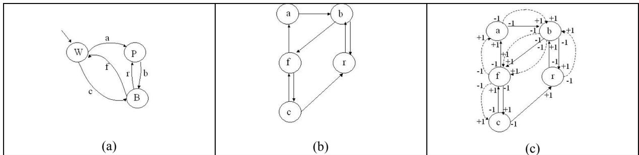
Figure 2. Condado algorithm. (a) FSM example; (b) Dual graph with arcs; (c) "Eulerized" Graph.
